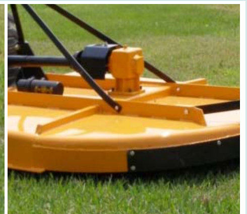
Heavy Duty Gearbox (field rated @ 65HP)
